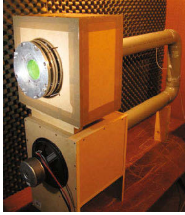
Figure 3. Photograph of the set-up. The membrane (in green) is supported by a device that allows to change the diameter and the pre-stress.
