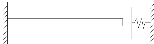
Figure 17. Clamped-free bar with an unilateral contactor at one end.
