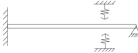
Figure 22. A clamped-simply supported beam with a bilateral contactor.
